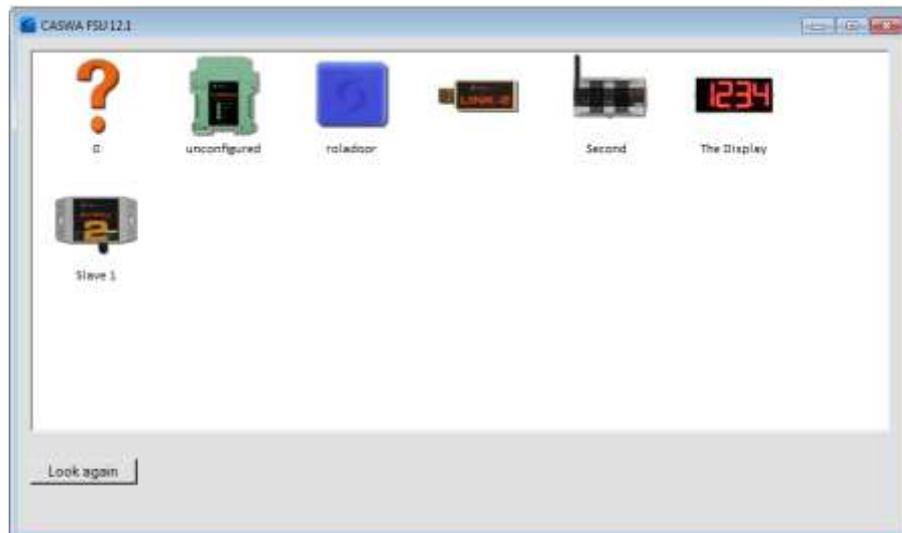
Series 2 AirWay devices are shown with a '2' over the AirWay icon. Series 1 devices do not have a number.
